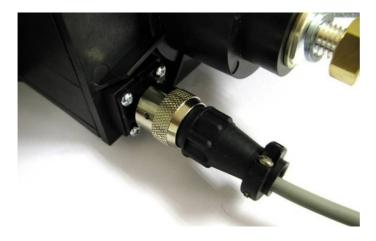
The 3 pole connector mounted on the rear is connected to a micro-switch inside the unit that is activated only when all connectors are in place and the unit is locked.
