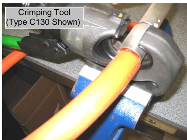
**Figure 7. Example Of Crimp Operation**
