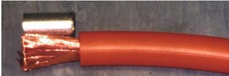
**Figure 10. Showing Cable Stripped Alongside Reduction Sleeve**
